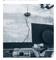
SGS provides effective inspection solutions for difficult-to-access tank walls and roofs and other remote locations. The (semi)motorised tank wall scanner can climb carbon steel tank wall with magnetic wheels. It can carry out several remote inspections:
